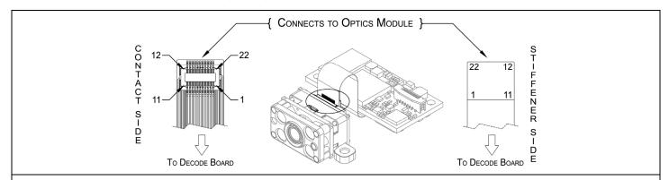
Figure 36. Flex Cable Pinout (Imaging Engine Connector End)
